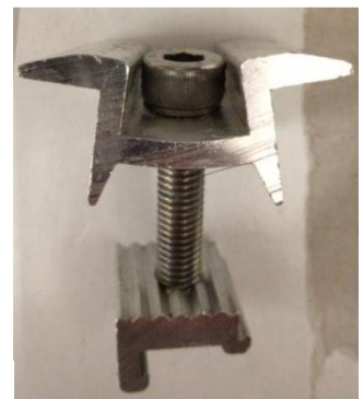
Deformation of mid-clamp caused by excessive torque
