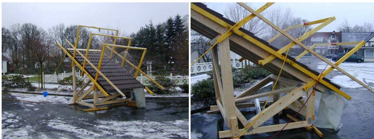
**Illustration 6: different directions of irrigation of the 30° inclined reference surface area.**
