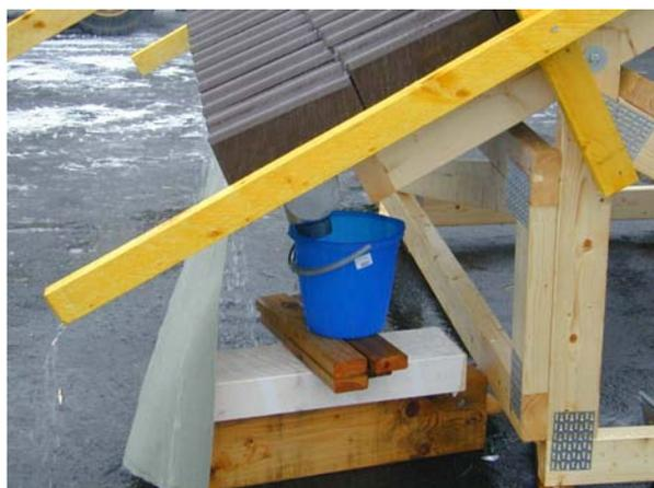
In the end it was stated that no water had penetrated the covering, both the rain water drain and the collector bucket remained free of water.
