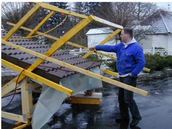
After the end of the test the roof surface area was irrigated by hand with a water hose for about 2 minutes (see illustration above), in order to find out, how the covering reacted to extreme conditions. The quantity of water collected of about 100 ml was quite remarkable in view of the short duration.
